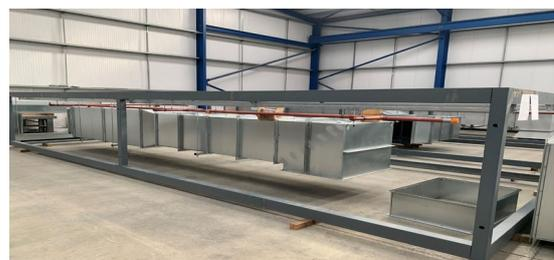
Fig 1.2 Plant Room elements in Production.
